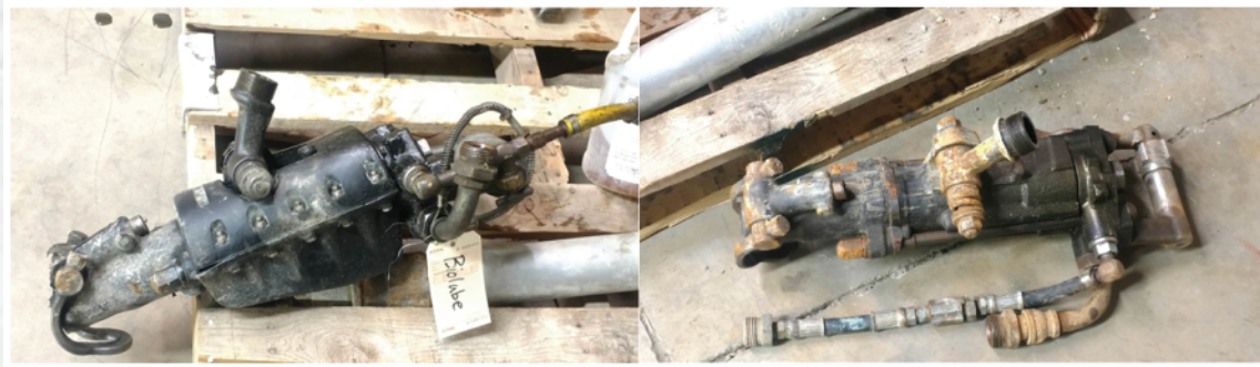
Pictured above: (Left) Jackleg drill using BioLube RD (Right) Jackleg drill using conventional oil.
