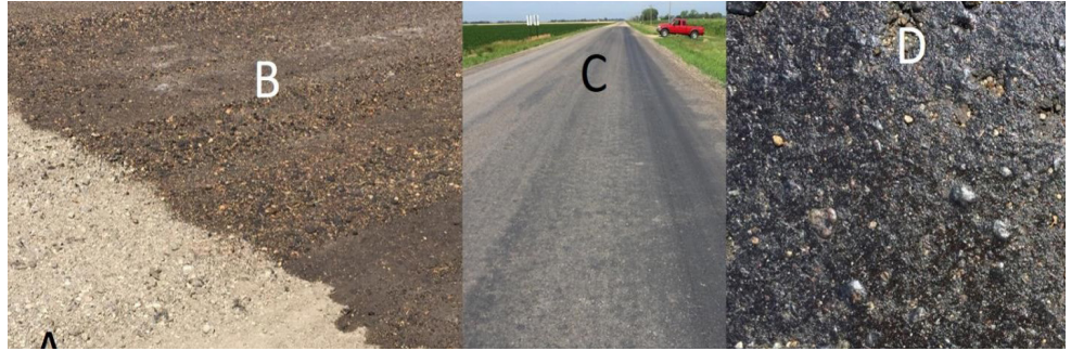
A) Untreated gravel. B) 30 minutes after treatment. C) After 6 weeks D) Close up of treated road surface. (Actual test conducted on gravel with a 25% asphalt regrind mixture).
